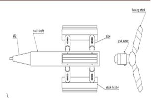
Fig: 5. Honing tool for a drilling machine
