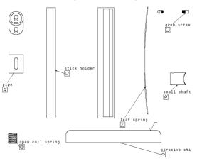
Fig: 6. Different parts of a honing tool Table: 1. Parts List
